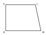
3. Investigate: Use strips and fasteners to make a triangle and a quadrilateral. Try to push inward at any one vertex of the triangle. Do the same to the quadrilateral. Is the triangle distorted? Is the quadrilateral distorted? Is the triangle rigid? Why is it that structures like electric towers make use of triangular shapes and not quadrilaterals?
